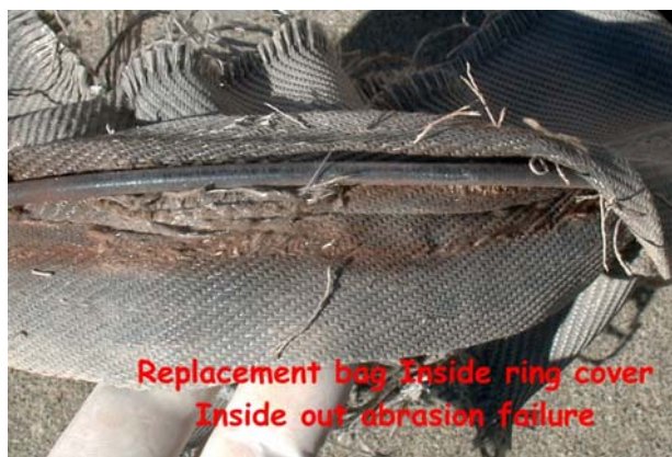
Figure 5 – Bag Ring Corrosion
