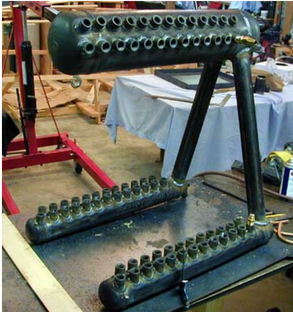
Welded Steel Pressure Vessel
