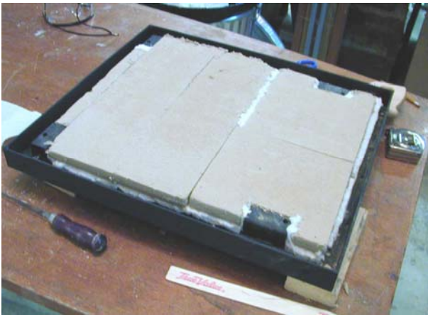
Boiler Base with Insulation
