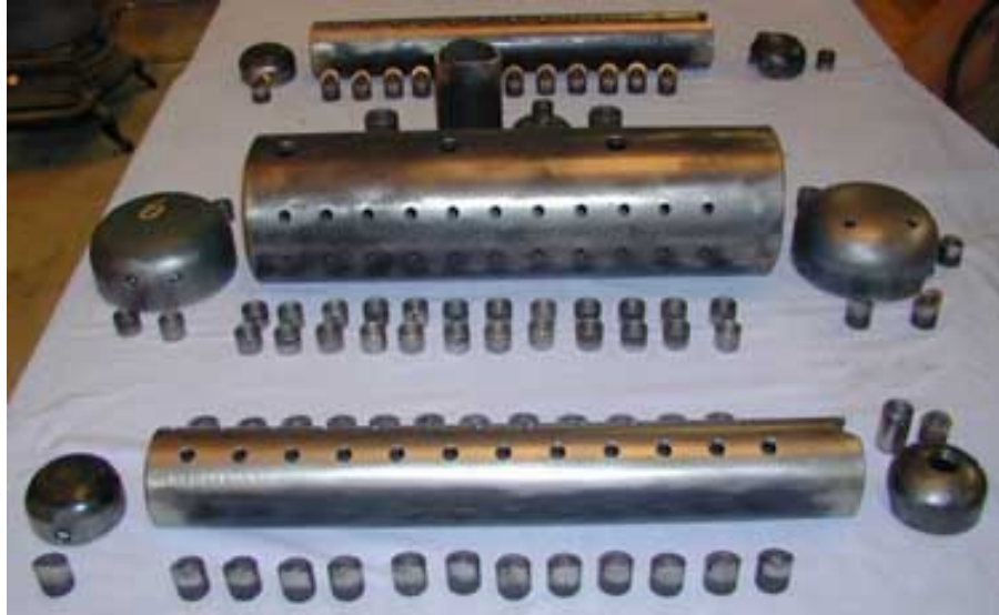
Boiler Parts Prepped and Ready To Weld
