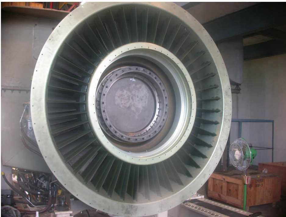
VIGV in fully open position
