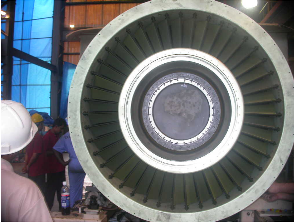
VIGV in fully open position
