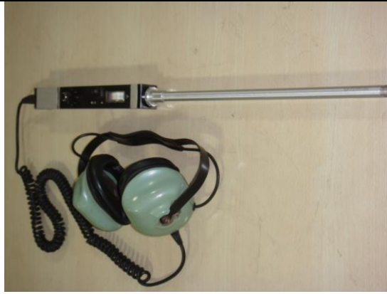
Ultrasonic leak detector being used for compressed air leak survey
