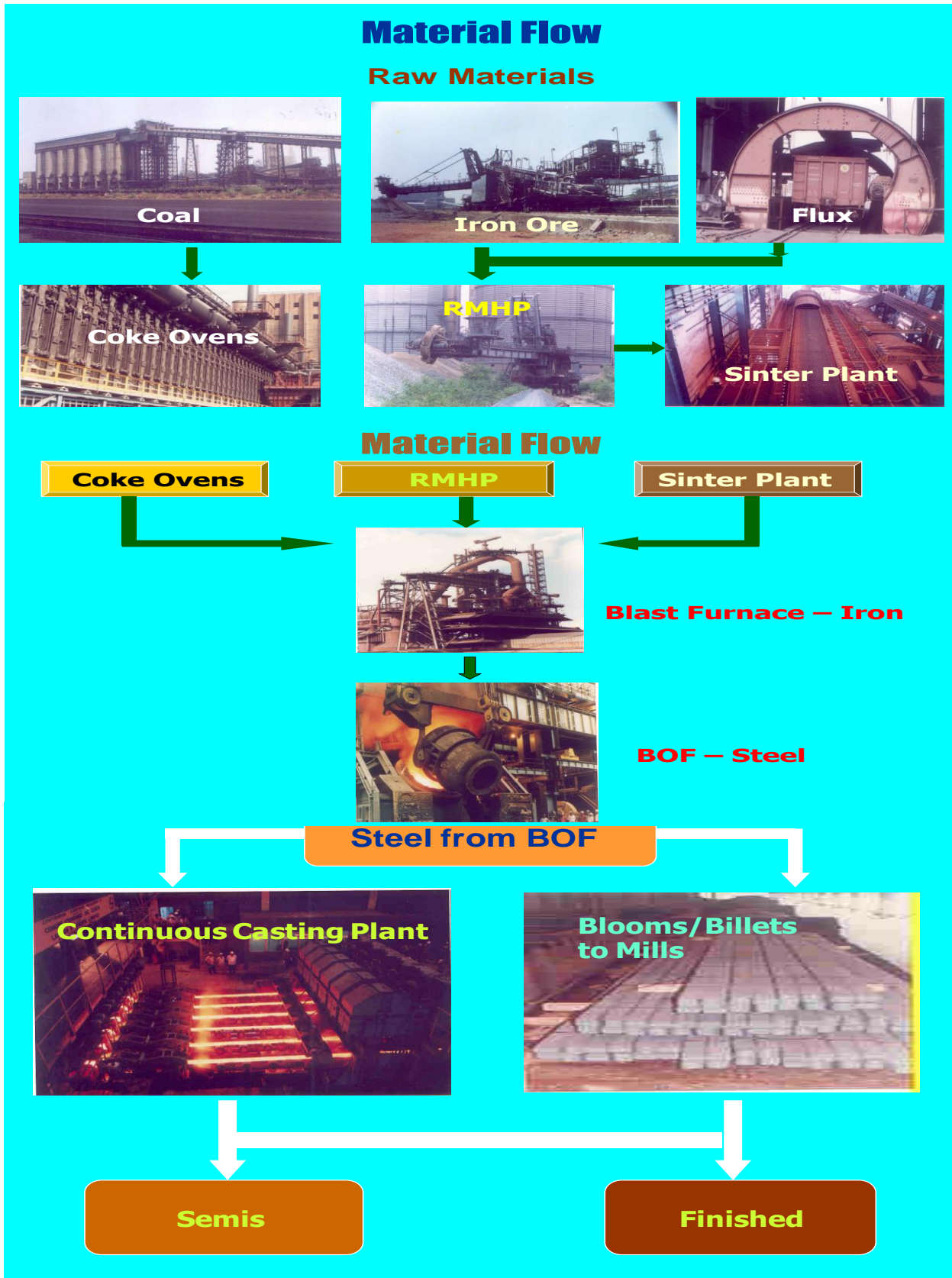
Figure 1. PROCESS FLOW CHART: DURGAPUR STEEL PLANT
