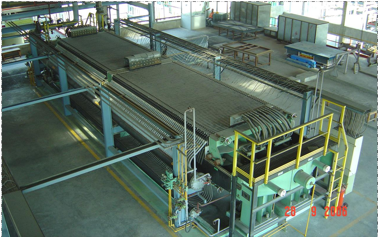
View -----> NCH type of electrolyser – Next higher version of NCS type of electrolyzers.
