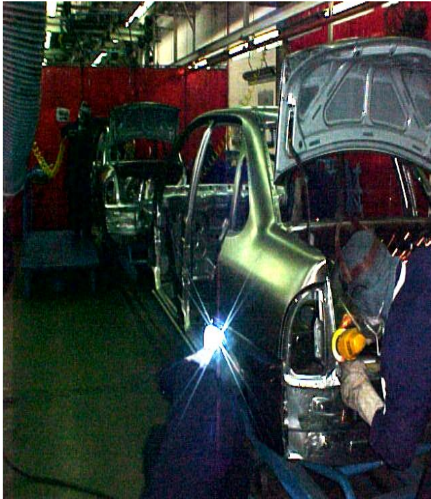
Door panel welding
