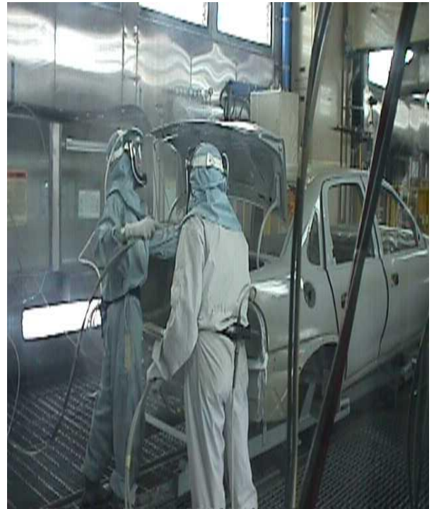
Primer coat - Utility cabin painting
