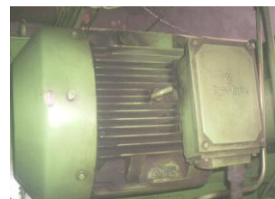
50 HP Motor for vertical broaching machine
