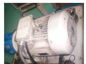
5 HP motor for hydraulic press.
