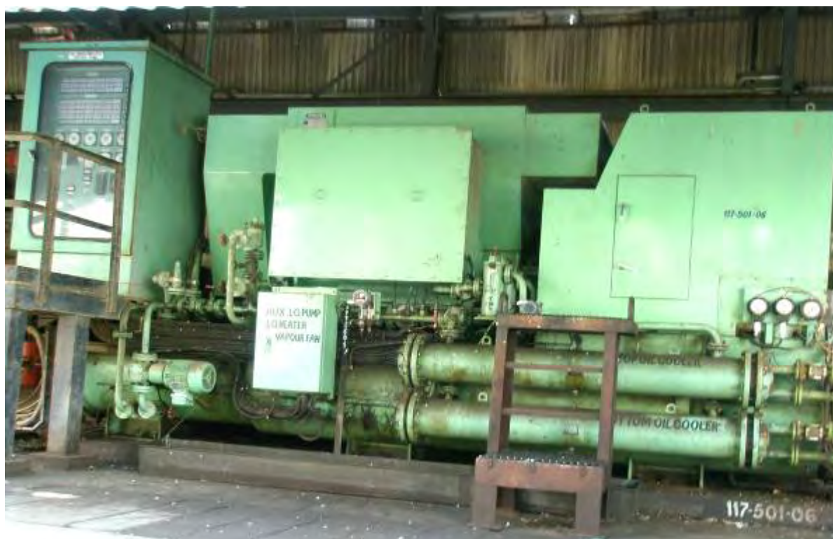
(Photograph showing Mitsubishi Air Compressor for which overhaul job was carried out for improving Energy Efficiency and performance)
