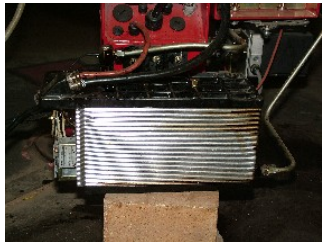
FO heater for burner
