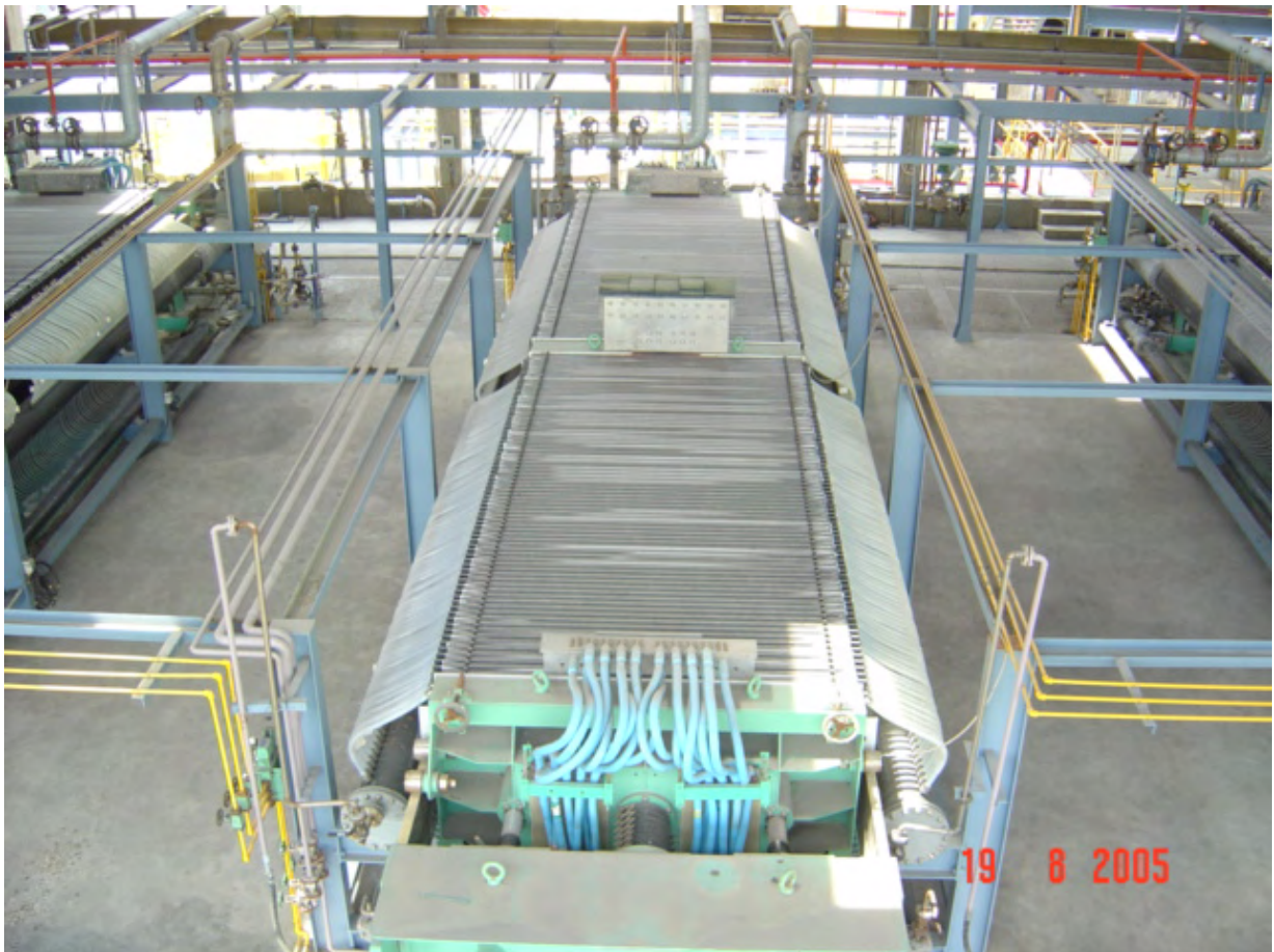
View---> Natural circulation NCS type of electrolysers
