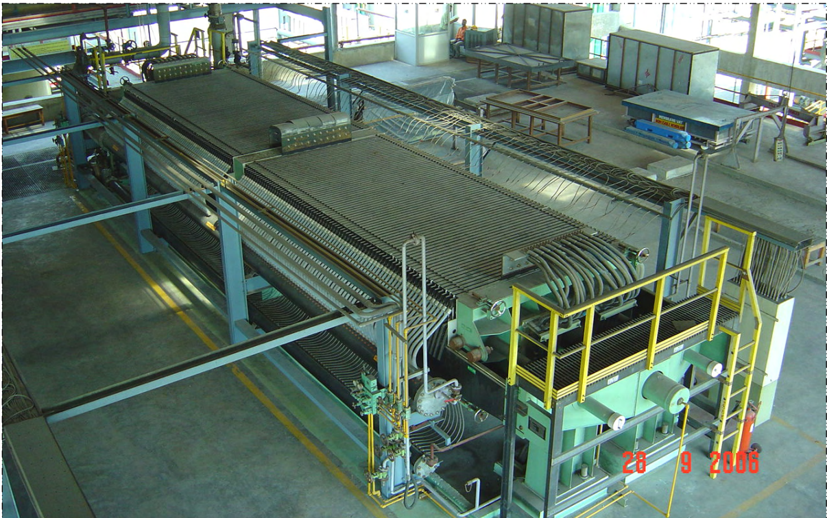
View -----> NCH type of electrolyser – Next higher version of NCS type of electrolysers.
