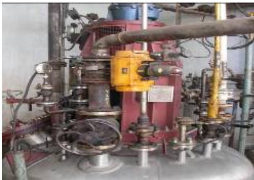
New Hydrogenation Reactor With Inside/Outside Limpet Coil
