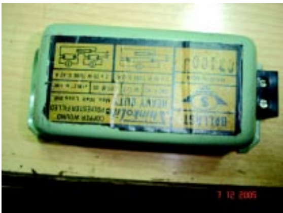
Copper chokes are being replaced in a phased manner
