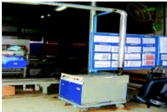
Electrical heating for generation of steam
