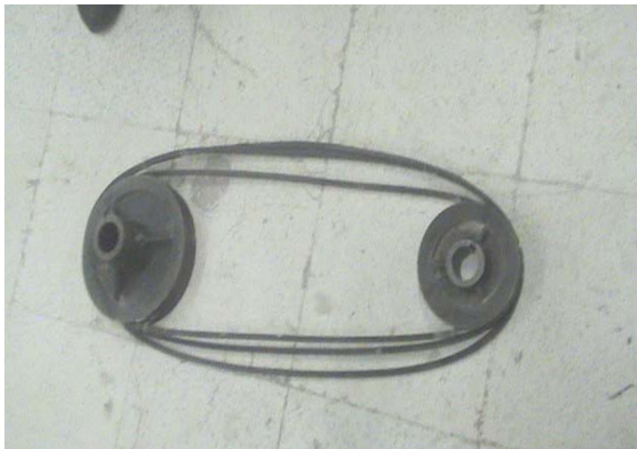
EARLIER INSTALLED V-BELTS ON MAIN SUCTION MOTOR ON WINDING MACHINES
