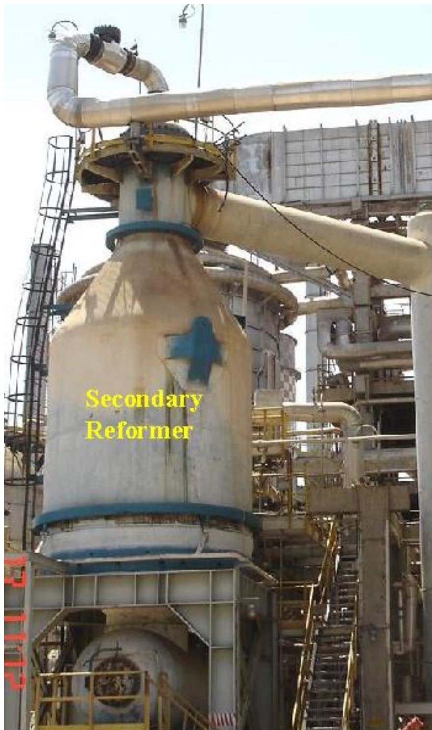
Fig-2: The secondary reformer where catalyst scooping was carried out.
