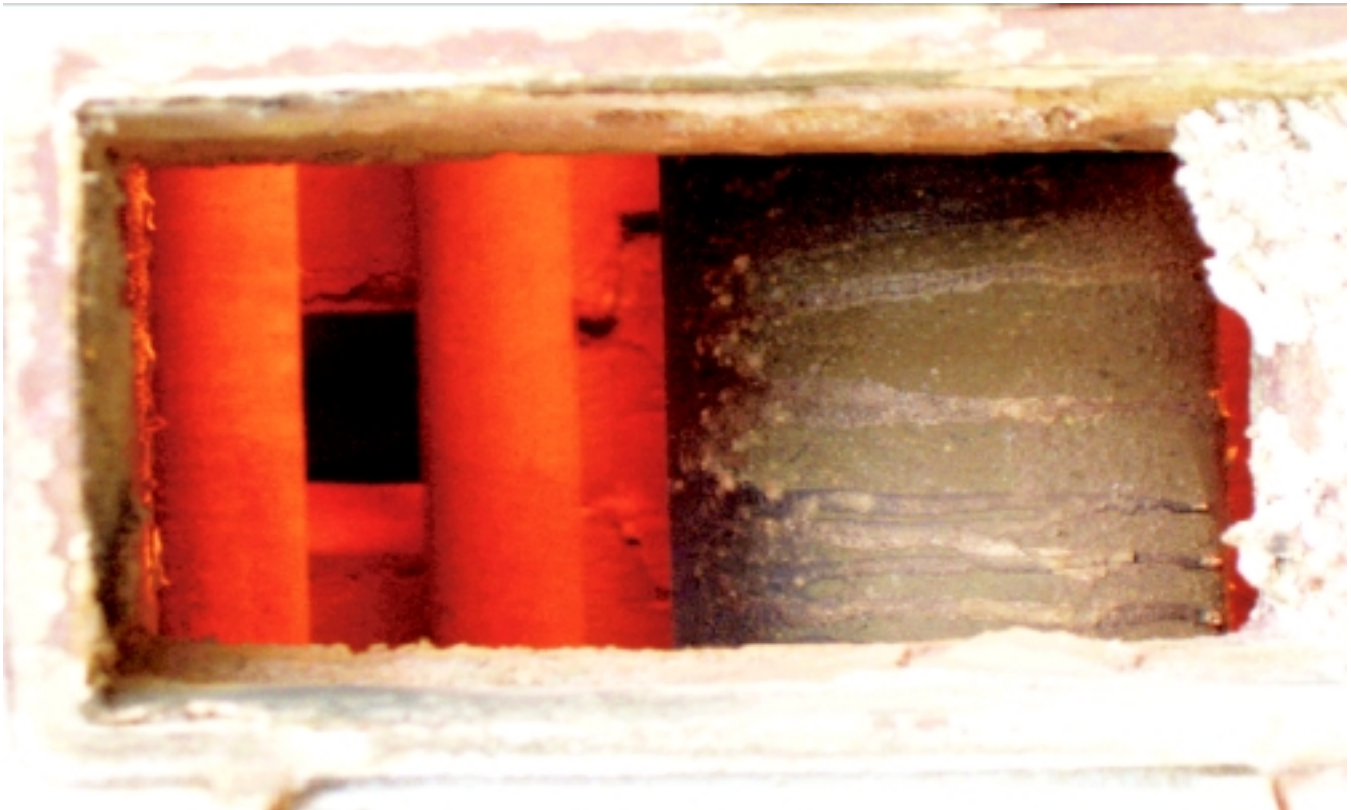
HIGH EMISSIVE CERAMIC COATING APPLIED ON THE REFRACTORY OF AU1 FURNACE FOR REDUCTION OF ENERGY CONSUMPTION
