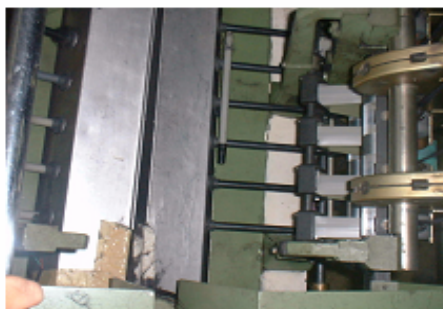
Double duct in Ring Frame Machine
