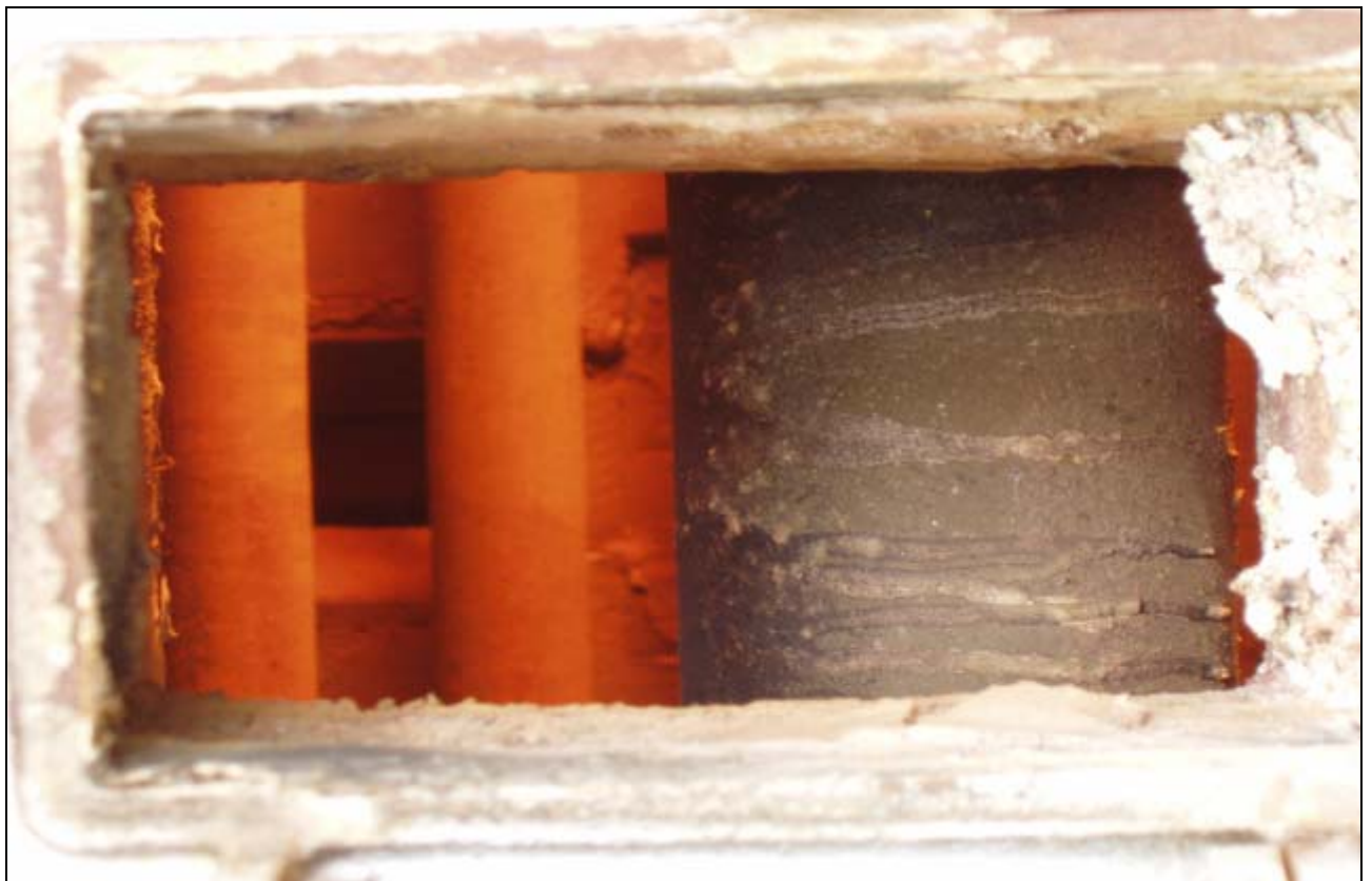
HIGH EMISSIVE CERAMIC COATING APPLIED ON THE REFRACTORY OF AU1 FURNACE FOR REDUCTION OF ENERGY CONSUMPTION
