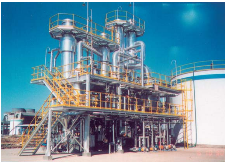
Membrane cell caustic concentration system
