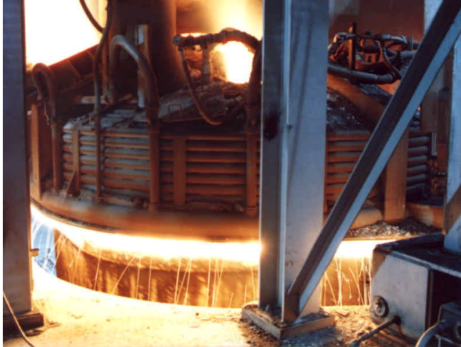
Ladle Metallurgy Furnace
