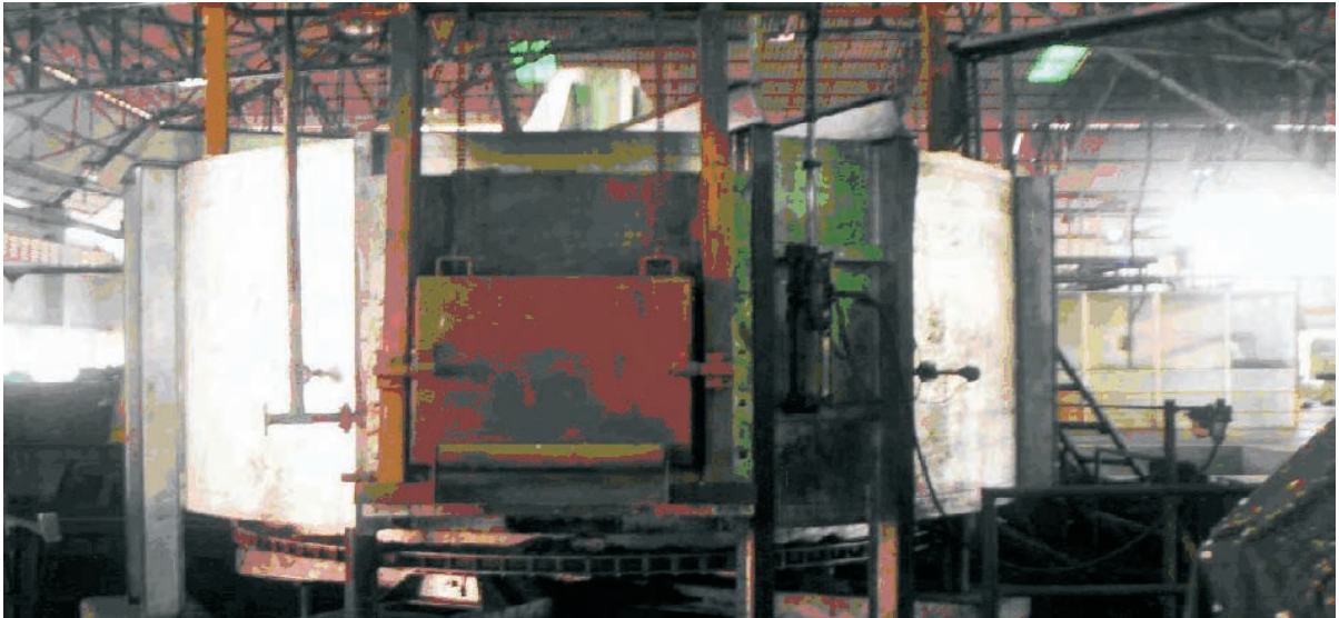
Rotary Furnace No.1 of 125 KW which is eliminated by C.G.C.F
