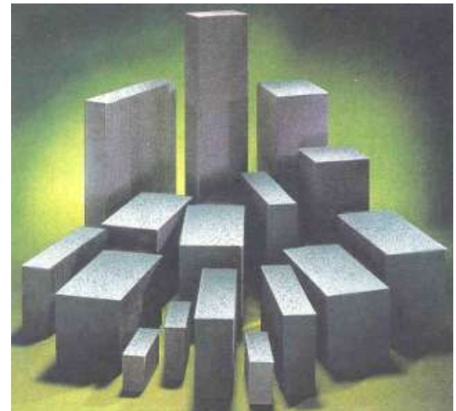
Aerated concrete blocks made of fly ash
