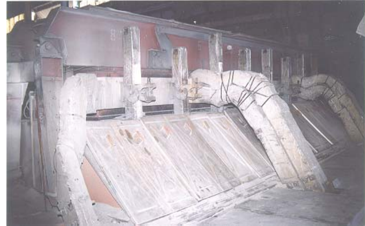
PHOTOGRAPH OF NALCO'S ELECTROLYTIC POT
