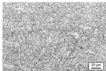
Tempered martensite, ≤ 2% δ-ferrite
